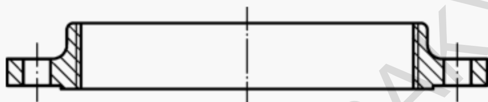
j) Type 13 Hubbed threaded flange
