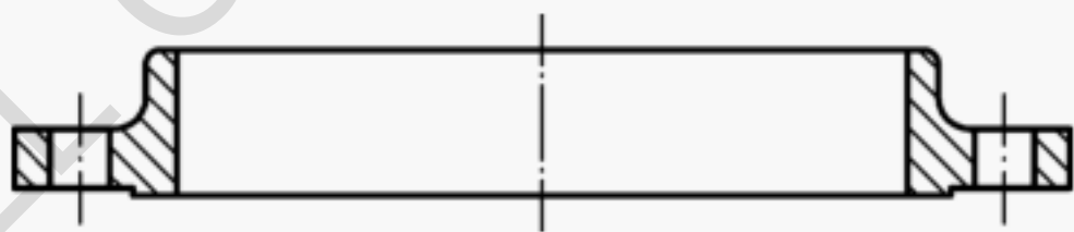
i) Type 12 Hubbed slip-on flange for welding
